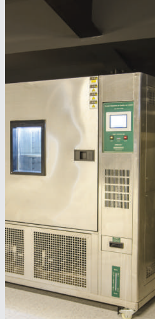
Isı, Nem Kabini Heat, Humidity Cabinets
